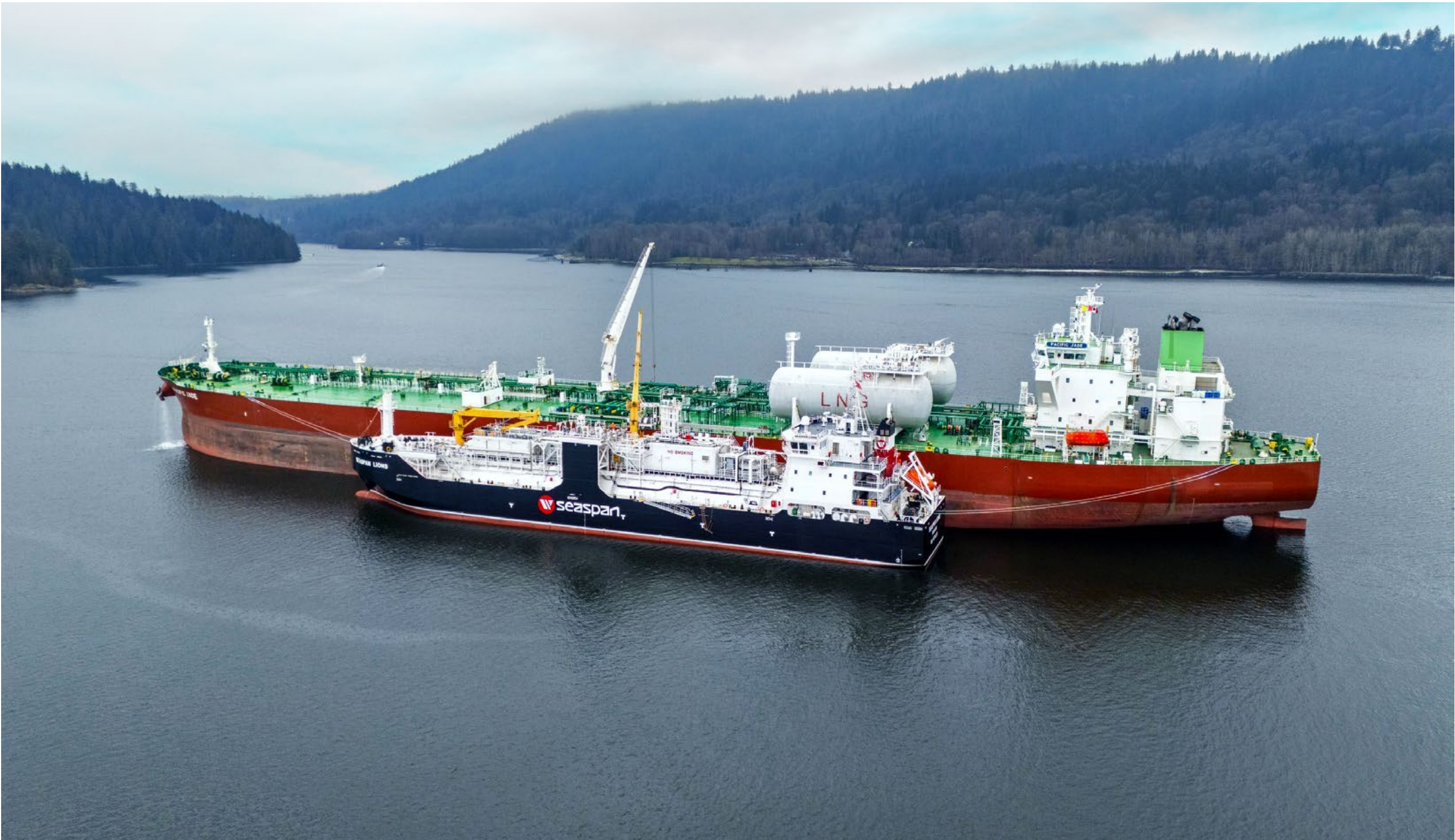
Seaspan Energy conducts ship-to-ship LNG bunkering in the Port of Vancouver.
