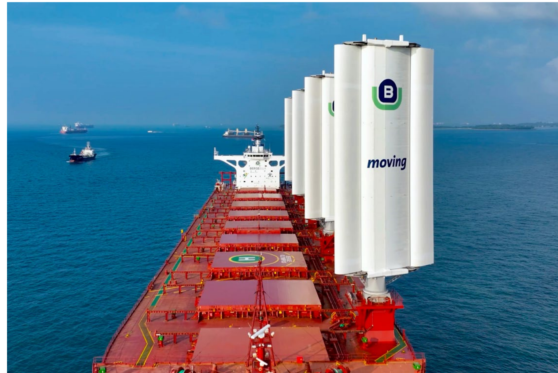
Berge Olympus, a bulk carrier equipped with four retrofitted wing sails.
