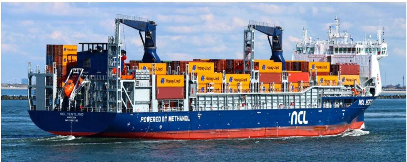
NCL Vestland, a methanol dual-fuel container feeder vessel.
